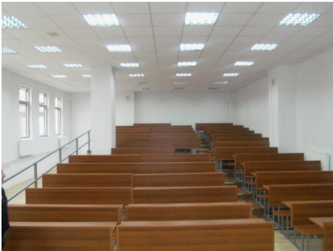
Figure 11-8 Refurbished lecture theatre at University Street site, Suspended ceiling grid, painted walls and polyvinyl flooring along with new furnishings, windows not replaced.
