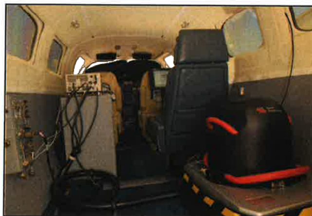
Leica ADS100 installation in a Surdex Cessna 441 (Conquest).
