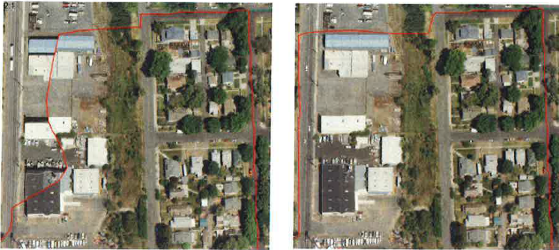
Initial automatic (left) and manually-adjusted (right) seamlines.
