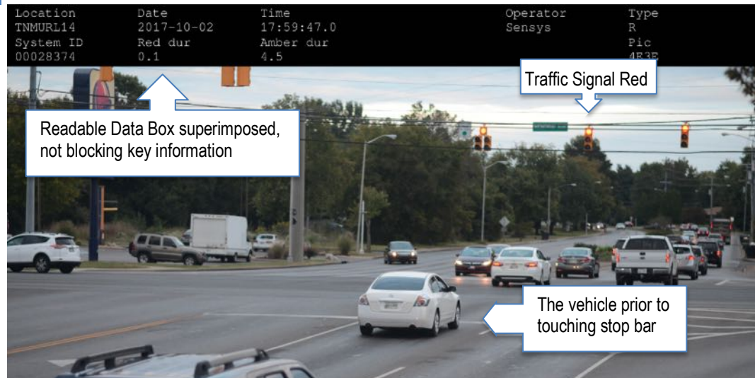
First Image in Color: Vehicle prior to stop bar, red phase signal, configurable data box superimposed not blocking info.
