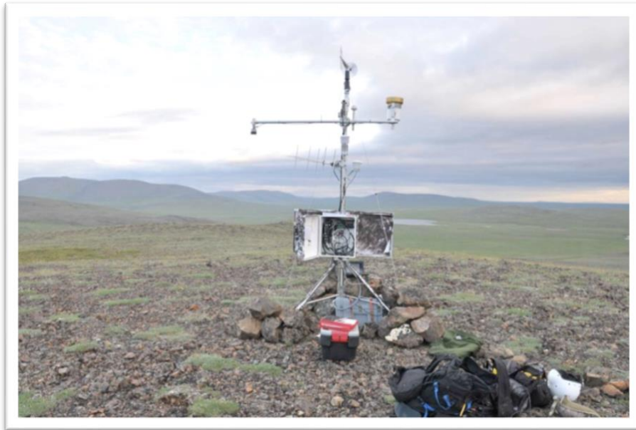
Figure 21: The Howard Pass RAWS station (courtesy DRI website). Snow depth sensor is on the arm projecting left. The gold-topped bucket is an unshielded precipitation gauge.
