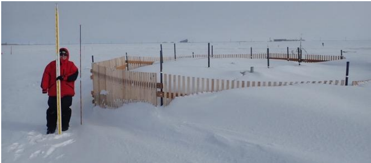
The Geonor precipitation gauge at Oliktok Point in April 2018, completely drifted over by the winter's heavy snow...but still sending out (erroneous) autonomous data.
