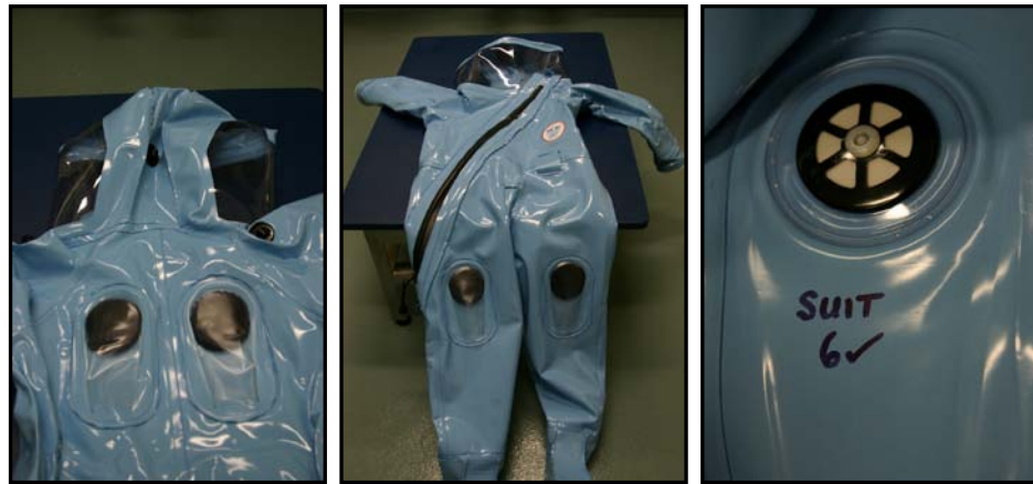
(All above) Multiple breathing air exhaust vents
